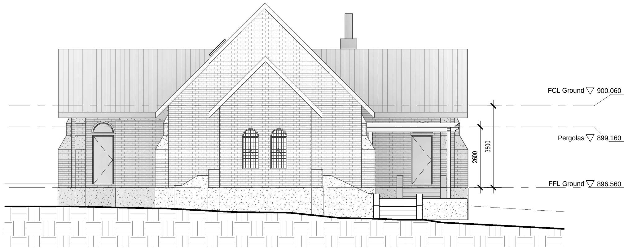
1 DA101 ELEVATION 1 : 100 EAST ELEVATION
